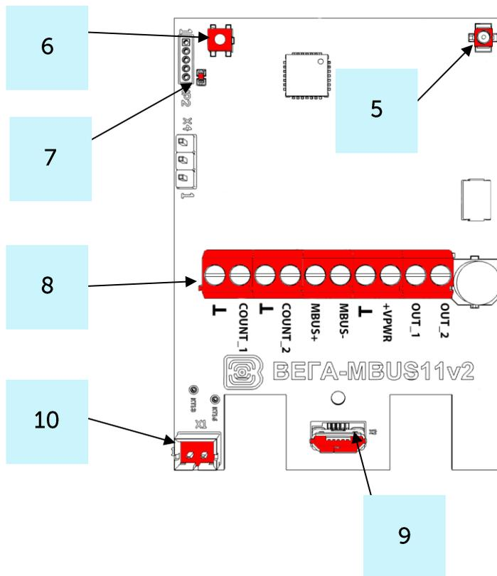
5 – input for connecting an external antenna
