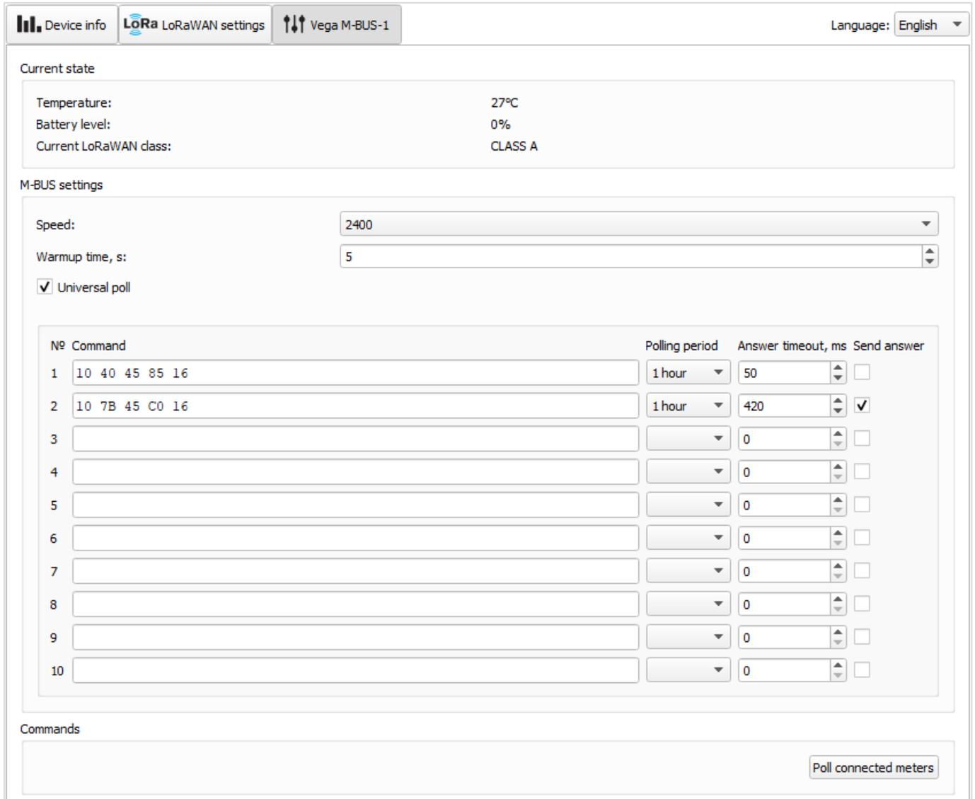
The screenshot shows the configuration interface for the Vega M-BUS-1 device. It includes tabs for 'Device info', 'LoRa LoRaWAN settings', and 'Vega M-BUS-1'. The 'Current state' section displays: Temperature: 27°C, Battery level: 0%, and Current LoRaWAN class: CLASS A. The 'M-BUS settings' section shows Speed: 2400, Warmup time, s: 5, and the 'Universal poll' checkbox checked. Below this is a table for configuring polling commands.
